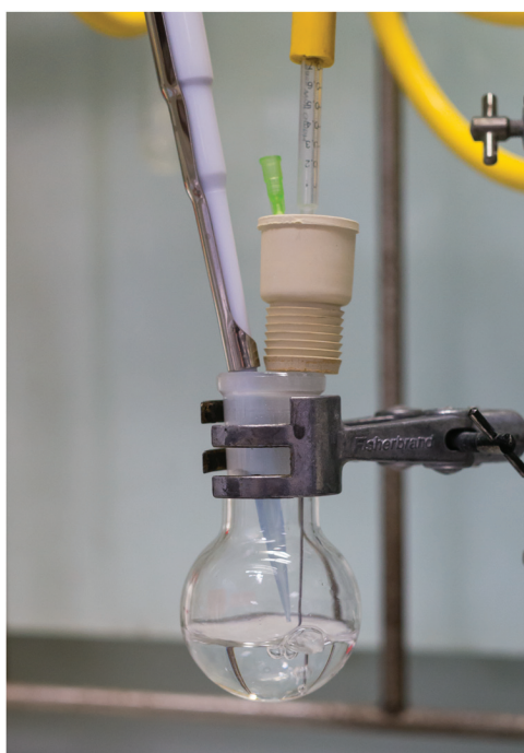
Figure 4 | Pipetting deoxygenated solvent from flask A into reagent vials.
