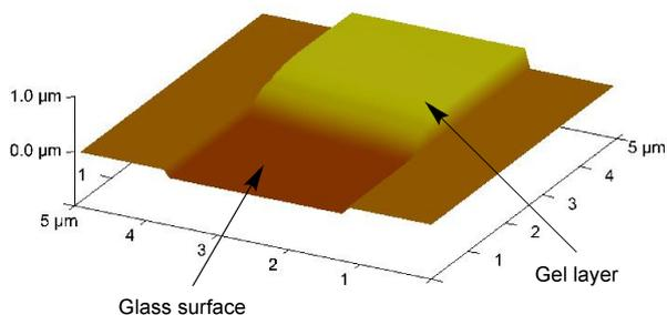
**Fig. 1** AFM 3D surface image of a 3D hydrogel slide, where the gel had been removed from part of slide by a scratch test. Average gel thickness across two different slides = 470 nm, based on average of three different cross-sectional measurements per slide (490 and 450 nm). See ESI† for further details.
