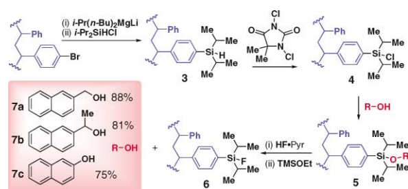
Scheme 3 Synthesis of diisopropylsilane-functionalized polystyrene ( 3 ) and its use for attaching primary, secondary and phenolic alcohols covalently onto the polystyrene solid-support. Overall yields from silane polystyrene 3 (three steps) were calculated by mass after cleavage of the alcohols from the polymer.
